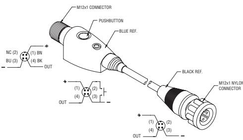
**AC132** Right-angle, M12 micro, 4-conductor, connector/cable assembly, 5 m (16') (for flat-profile connector-style sensors)
